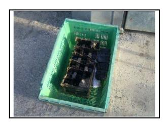
The top of this lorry battery exploded whilst it was under charge, resulting in injuries to an engineer's face and eyes
